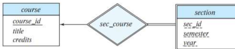
Figure 6.14 E-R diagram with a weak entity set.
